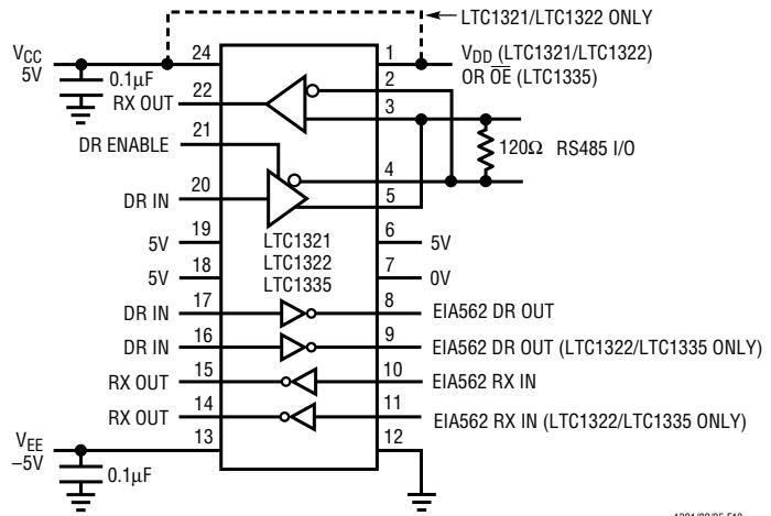
Figure 13. EIA562/RS485 Interfaces with  $\pm 5V$  Supplies
