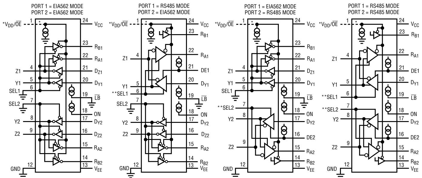
\* FOR LTC1322 ONLY, PIN 1 IS V<sub>DD</sub>, AND OE IS ALWAYS ENABLED.
