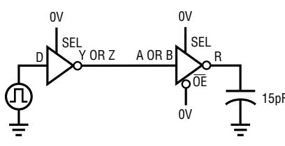
Figure 5. EIA/TIA-562 Receiver Timing Test Circuit
