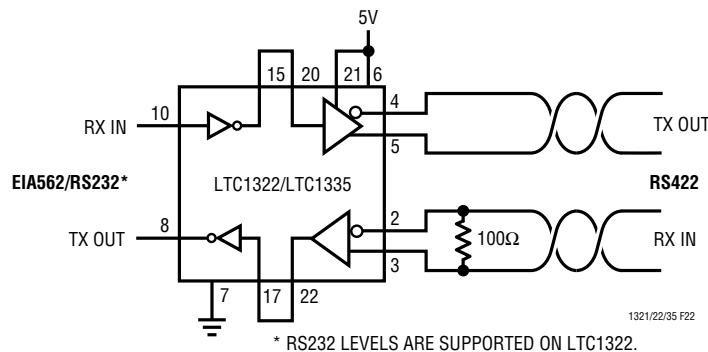
Figure 22. Typical EIA562/RS232 to RS422 Level Translator
