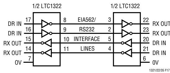
Figure 17. Typical Connection for EIA562/RS232 Interface
