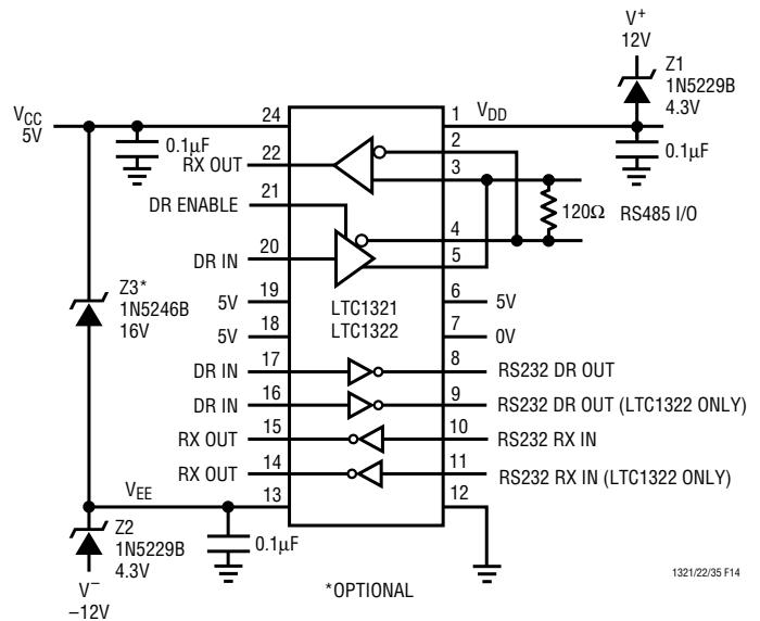
Figure 14. RS232/RS485 Interfaces with 5V,  $\pm 12V$  Supplies
