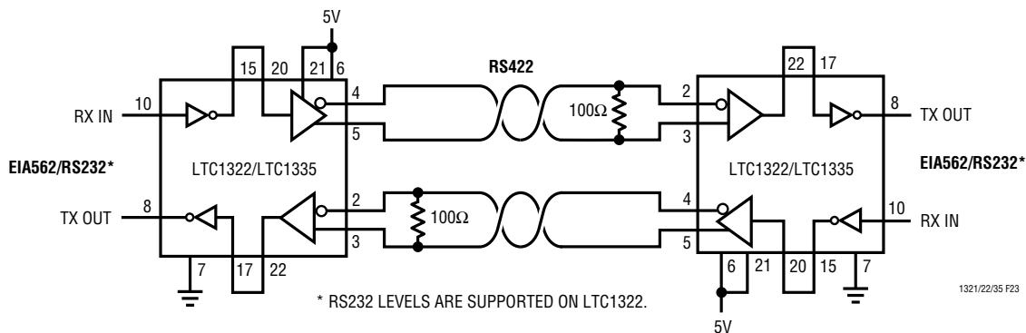
Figure 23. Typical Cable Extension for EIA562/RS232 Interface
