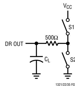
Figure 3. RS485 Driver Output Enable/Disable Timing Test Load
