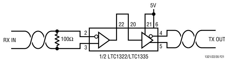
**Figure 21. Typical Cable Repeater for RS422 Interface**
