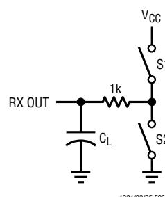
Figure 6. Receiver Output Enable/Disable Timing Test Load
