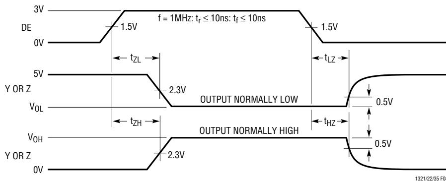
Figure 8. RS485 Driver Enable and Disable Times
