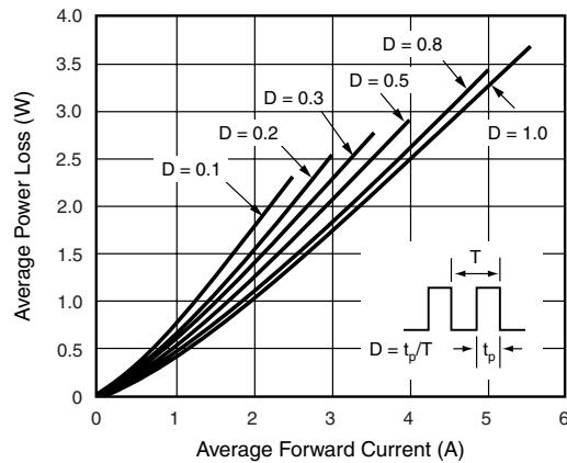
Figure 3. Forward Power Loss Characteristics Per Diode
