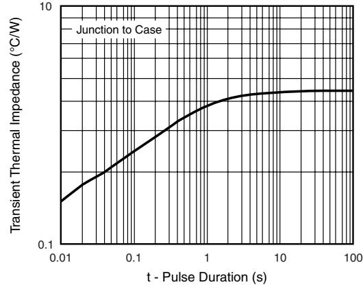
Figure 7. Typical Transient Thermal Impedance Per Diode
