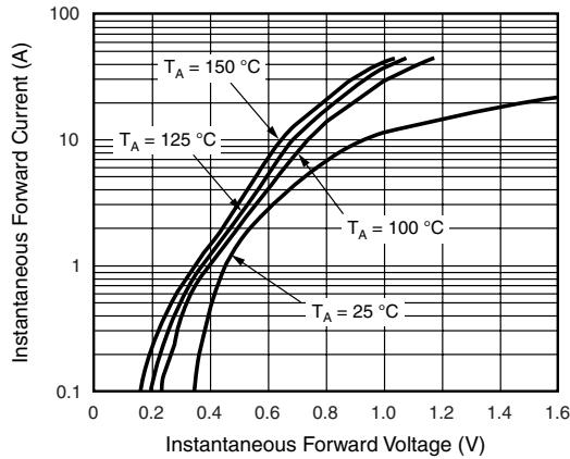
Figure 4. Typical Instantaneous Forward Characteristics Per Diode
