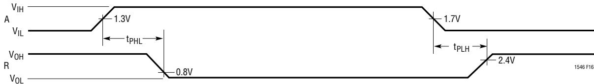
Figure 16. V.28 Receiver Propagation Delays
