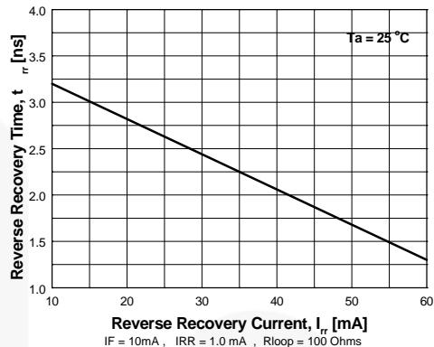
**Figure 8. Reverse Recovery Time vs. Reverse Recovery Current**
