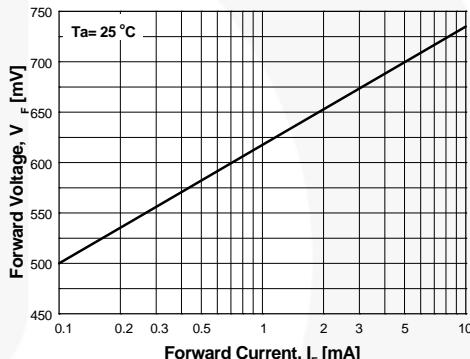
**Figure 4. Forward Voltage vs. Forward Current**
