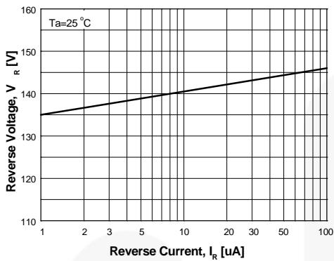
**Figure 1. Reverse Voltage vs. Reverse Current**
