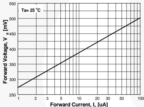
**Figure 3. Forward Voltage vs. Forward Current**
