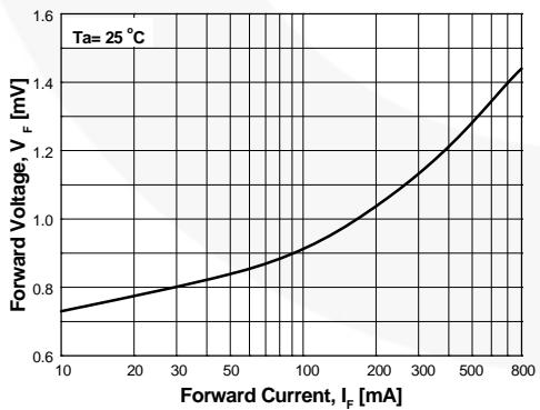
**Figure 5. Forward Voltage vs. Forward Current**
