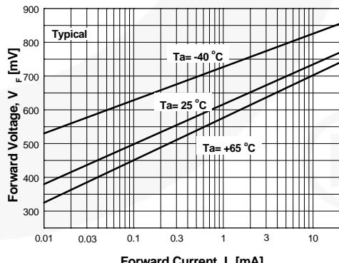
**Figure 6. Forward Voltage vs. Ambient Temperature**
