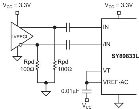
**Figure 3d. AC-Coupled LVPECL Input Interface**
