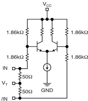
**Figure 1. Simplified Differential Input Buffer****LVDS OUTPUTS**
