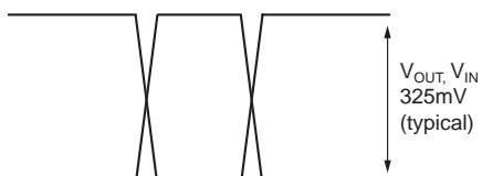
**Figure 2c. Single-Ended Swing**
