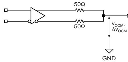
**Figure 2b. LVDS Common Mode Measurement**
