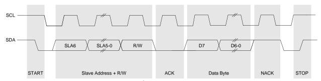
Figure 12. I<sup>2</sup>C Bit Timing Diagram
