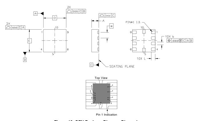
Figure 19. QFN Package Diagram Dimensions
