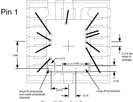
Figure 20. Photodiode Centers
