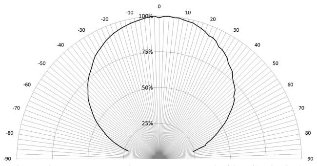
Figure 5. View angle, large photodiode rotated around the pin-5/pin-10 ("vertical") axis
