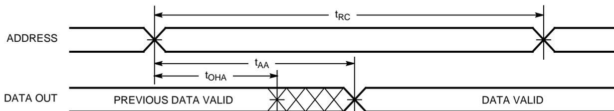
Figure 2. Read Cycle No. 2 ( $\overline{OE}$  Controlled) [15, 16]
