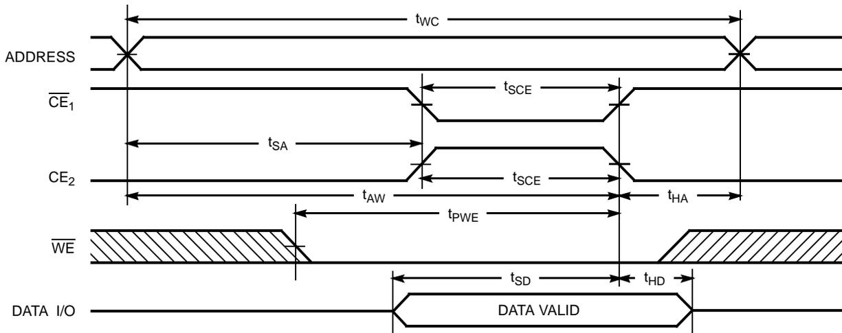
Figure 4. Write Cycle No. 2 ( $\overline{WE}$  Controlled,  $\overline{OE}$  HIGH During Write) [17, 18]
