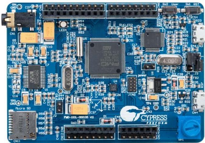
The FM0-100L-S6E1B8 MCU Starter Kit is a low cost development platform for Cypress's FM0+ S6E1B-Series, a Flexible Microcontroller family with an ultra-low-power 32-bit ARM® Cortex®-M0+ CPU. This kit enables rapid development of embedded systems with onboard interfaces including USB, micro SD Card and an Arduino™ Uno-compatible form-factor to prototype with Arduino shields.
