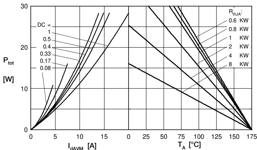
Fig. 4 Power dissipation vs. forward current
