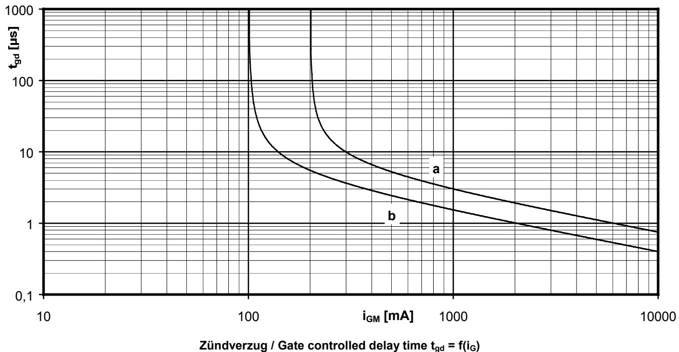
**Zündverzug / Gate controlled delay time  $t_{gd} = f(i_G)$**
