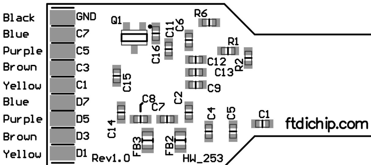
Figure 6.2 – UM232H-B-WE Wire Colours (Bottom View)
