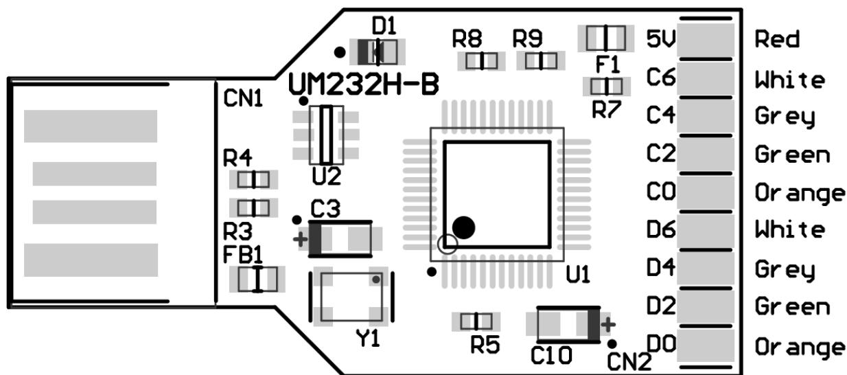
Figure 6.1 – UM232H-B-WE Wire Colours (Top View)
