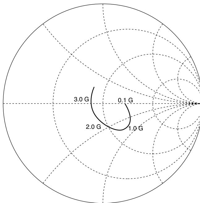
**TYPICAL S-PARAMETER VALUES ( $T_A = +25^\circ\text{C}$ )** $V_{\text{CC}} = V_{\text{out}} = 5.0 \text{ V}$ ,  $I_{\text{CC}} = 26 \text{ mA}$
