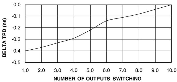
**DELTA T<sub>CO</sub> vs. # OF OUTPUT SWITCHING**
