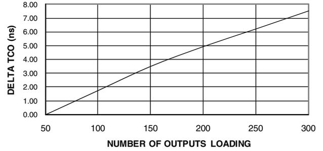
**DELTA T<sub>PD</sub> vs. # OF OUTPUT SWITCHING**
