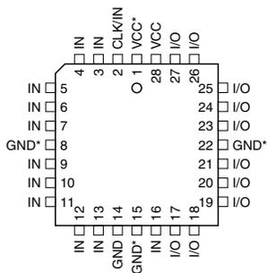
Note: For PLCC, P1, P8, P15 and P22 can be left unconnected. For superior performance, connect VCC to pin 1 and GND to 8, 15, and 22
