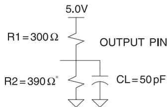
Note: Similar competitor devices are specified with slightly different loads. These load differences may affect output signals' delay and slew rate. Atmel devices are tested with sufficient margins to meet compatible device specification conditions.
