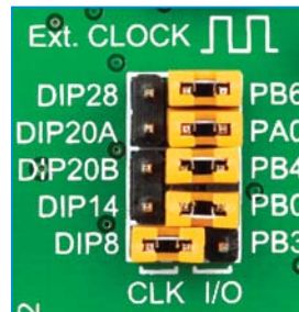
Figure 4-10: Position of the jumpers for DIP8
