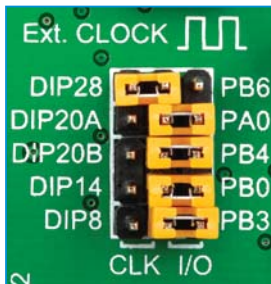
Figure 4-6: Position of the jumpers for DIP28
