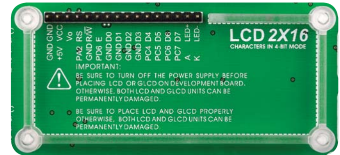
Figure 10-1: On-board LCD 2x16 display connector
