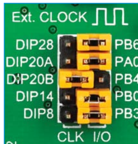
Figure 4-8: Position of the jumpers for DIP20B
