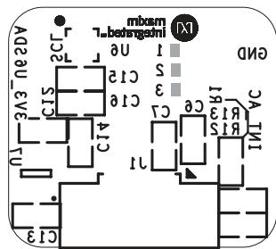
Figure 7. MAX30101 Daughter Board Component Placement Guide—Component Side
