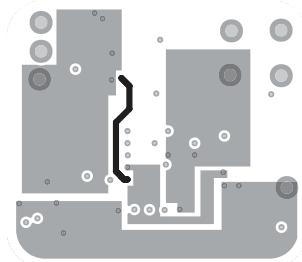
Figure 10. MAX30101 Daughter Board PCB Layout—Component Side
