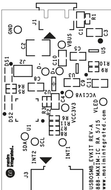
Figure 14. USBOSMB Mother Board Component Placement Guide—Component Side
