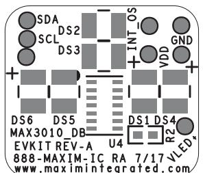
Figure 11. MAX30101 Daughter Board PCB Layout—Solder Side
