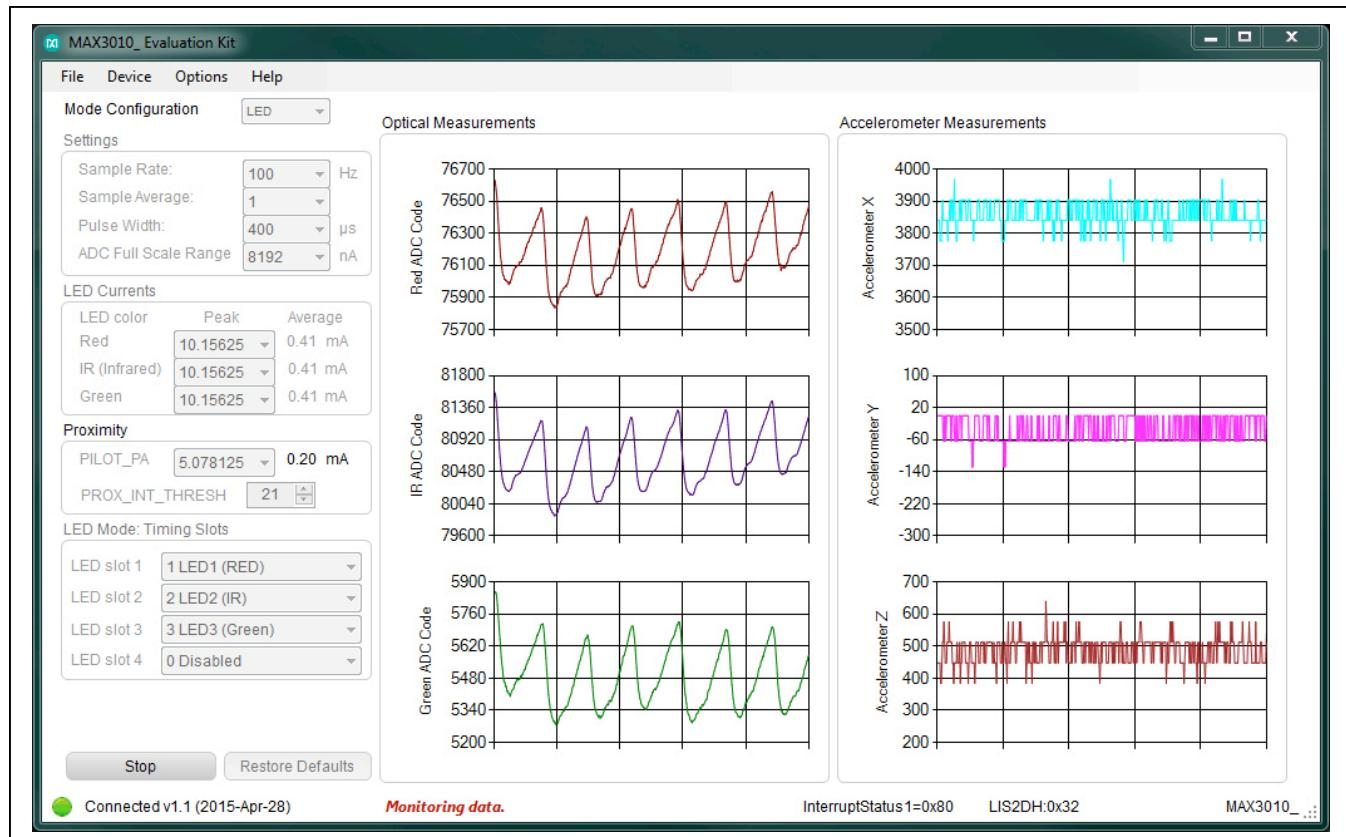
Figure 2. MAX30101 EV Kit Main Window (Sampling Data)
