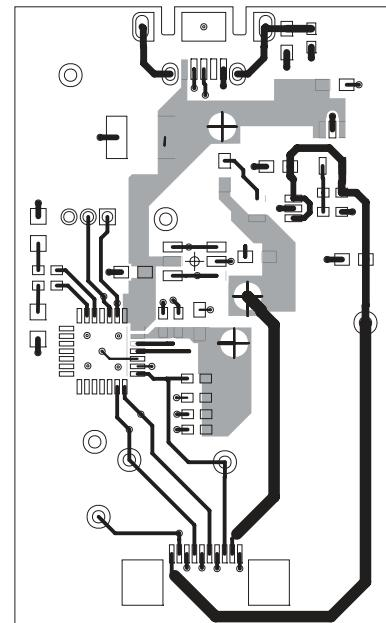
Figure 15. USBOSMB Mother Board PCB Layout—Component Side
