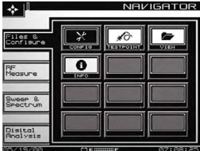
The Navigator user interface, common on all JDSU SDA meters
