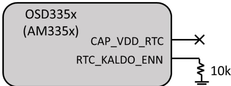
Figure 7.3. Additional connections for OSD335x with RTC enabled
