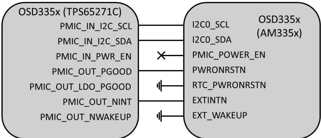
Figure 7.2. OSD335x Minimum Signal Connections with RTC disabled
