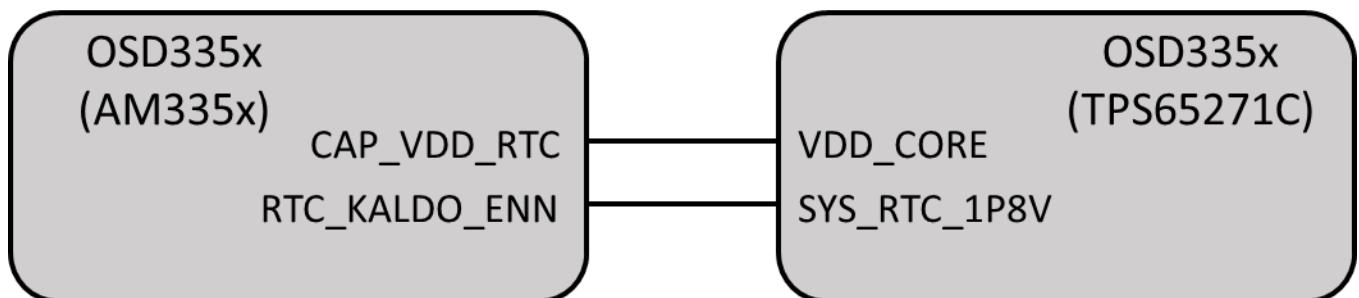
Figure 7.4. Additional connections for OSD335x with RTC disabled
