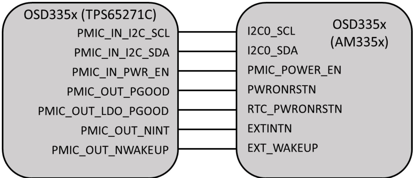
Figure 7.1. OSD335x Minimum Signal Connections with RTC enabled
