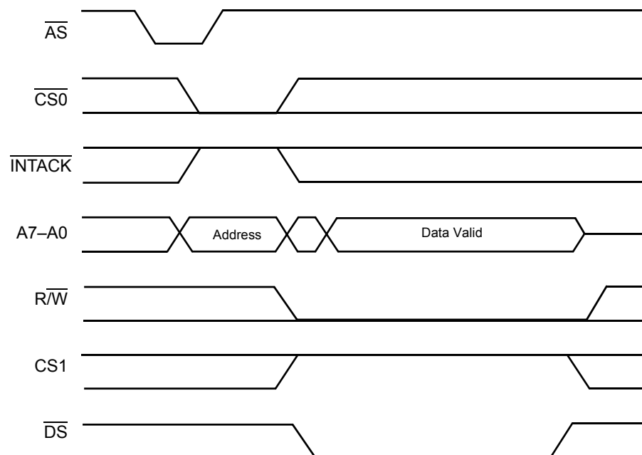
Figure 17. Z80230 Write Cycle Timing
