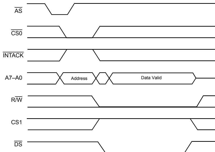
Figure 17. Z80230 Write Cycle Timing
