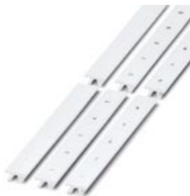
Zack marker strip, Strip, white, Labeled, Printed horizontally: L1, L2, L3, N, PE, Mounting type: Snap into tall marker groove, For terminal block width: 15.2 mm, Lettering field: 10.5 x 15.1 mm
