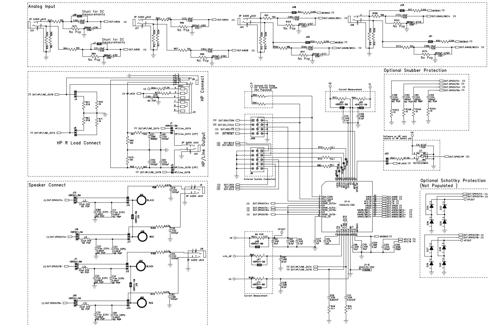
Figure 8. CS42L52 & Analog I/O (Schematic Sheet 1)
