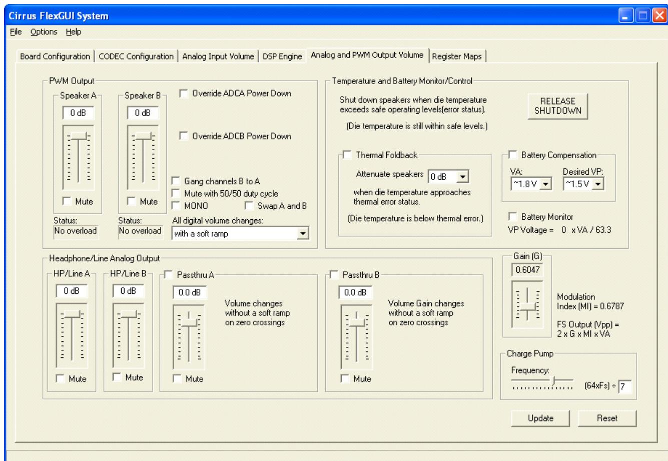
Figure 5. Analog and PWM Output Volume Tab
