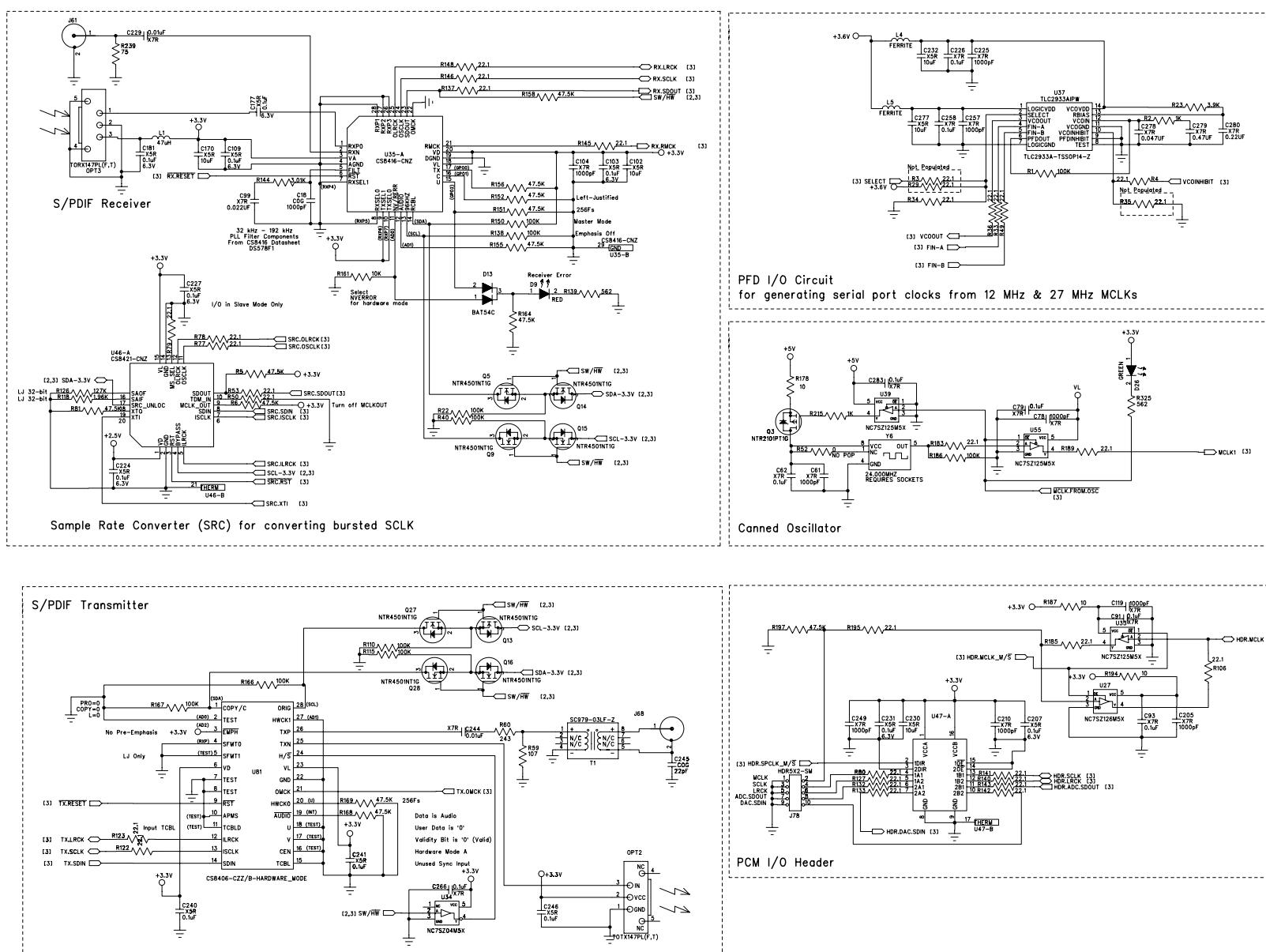
Figure 9. S/PDIF &amp; Digital Interface (Schematic Sheet 2)
