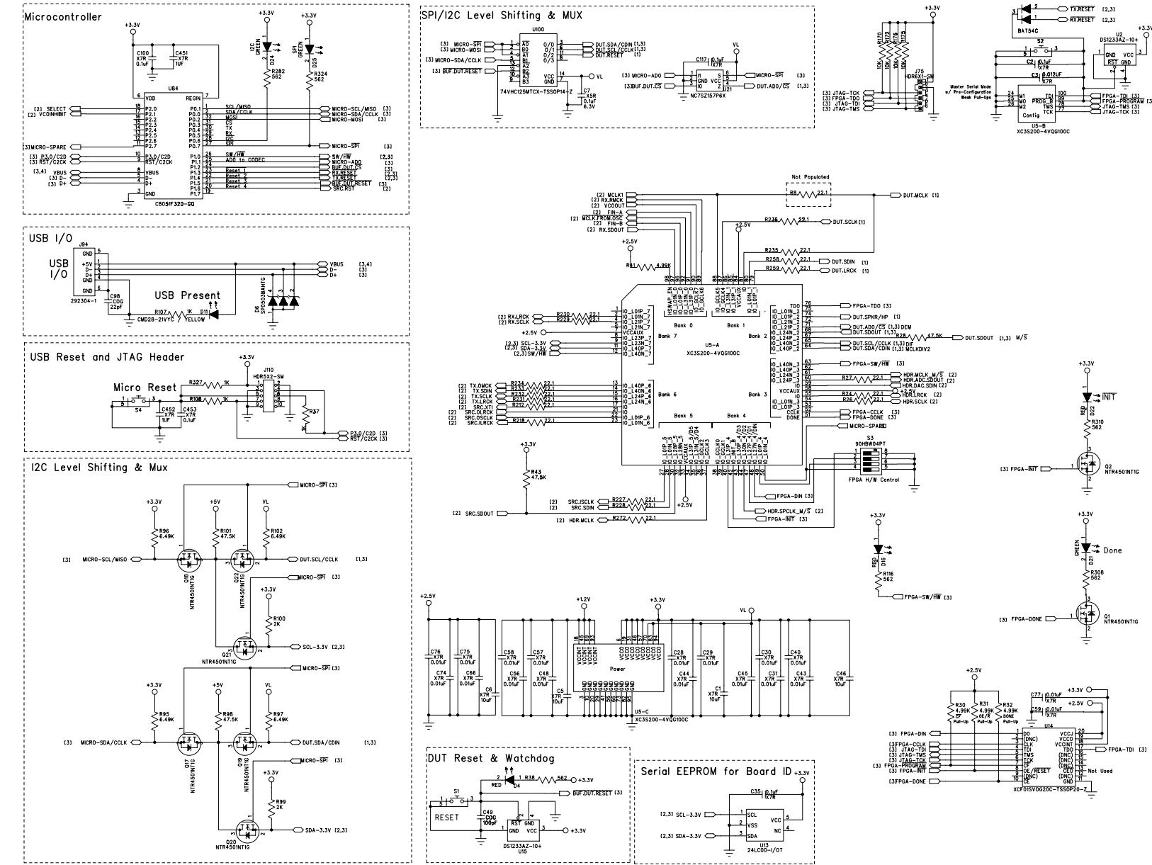
Figure 10. Micro &amp; FPGA Control (Schematic Sheet 3)
