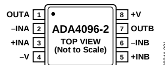
Figure 1. 8-Lead, MSOP (RM-8), ADA4096-2
