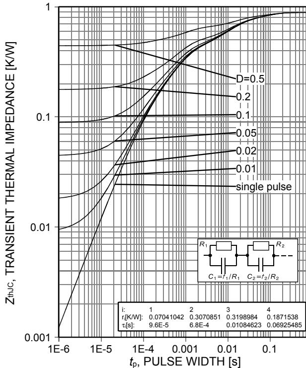
Figure 21. IGBT transient thermal impedance
