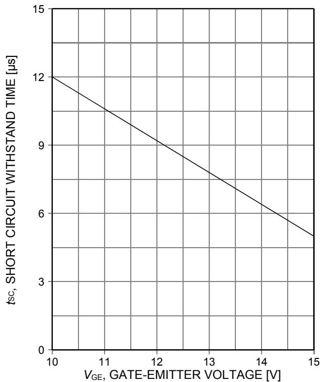
Figure 20. Short circuit withstand time as a function of gate-emitter voltage
