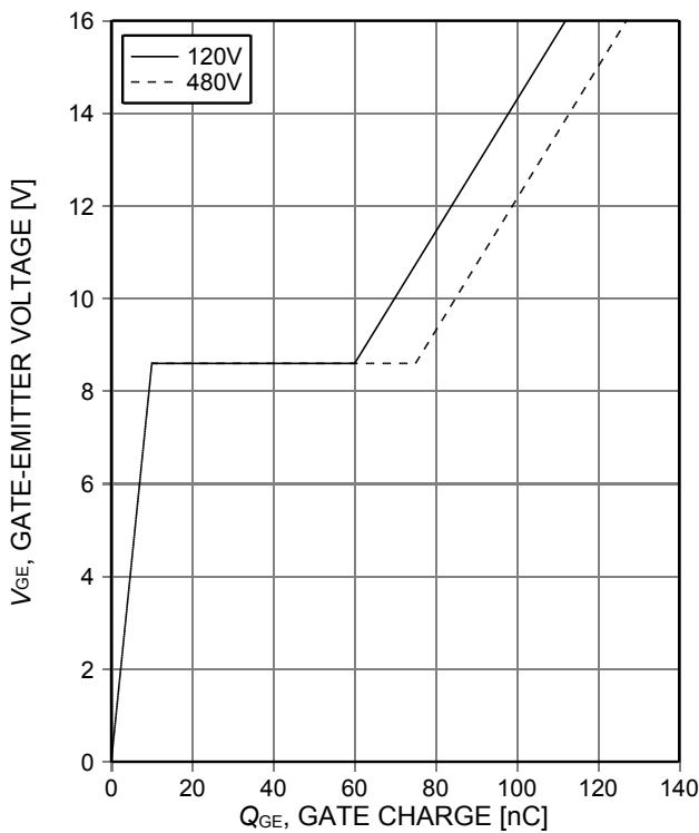
Figure 17. Typical gate charge
