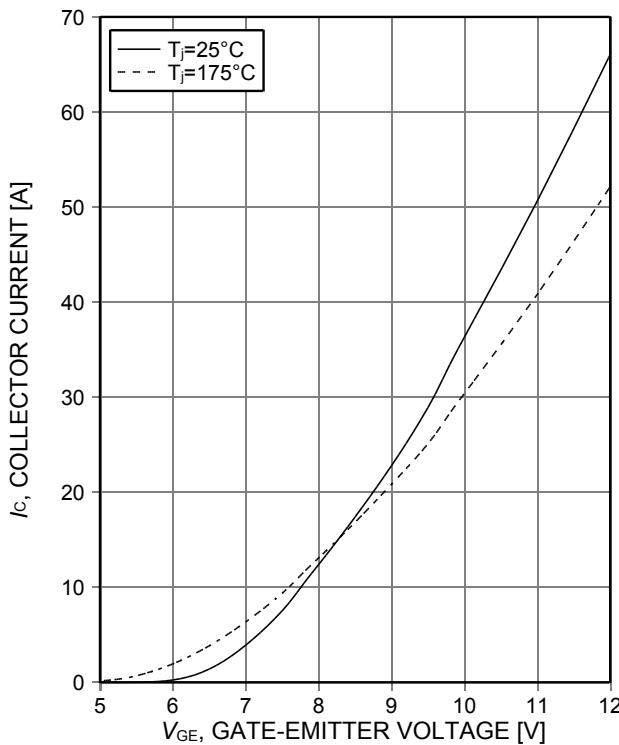
Figure 7. **Typical transfer characteristic**
