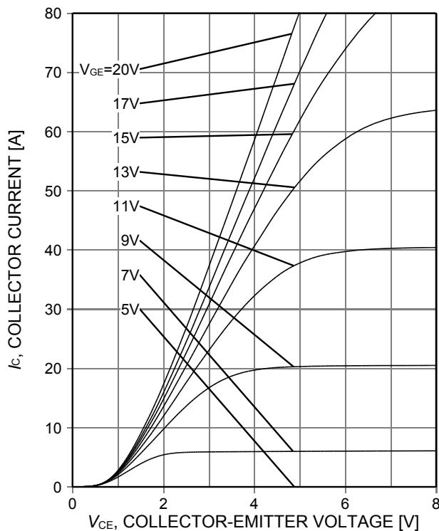
Figure 6. **Typical output characteristic**
