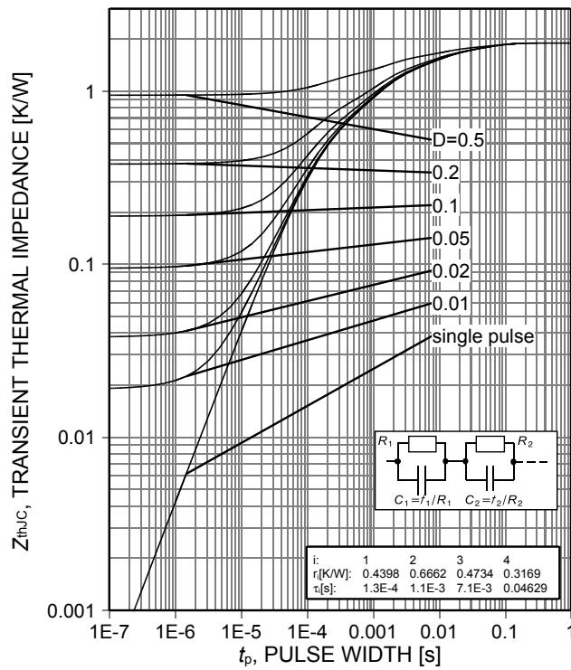
Figure 22. Diode transient thermal impedance as a function of pulse width
