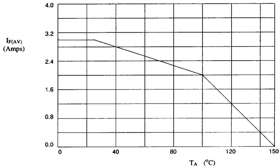
Fig 2. Maximum average forward current against ambient temperature.
