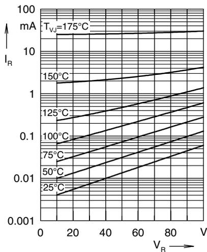
Fig. 2 Typ. reverse current  $I_R$  versus reverse voltage
