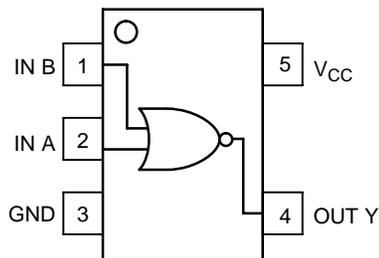
Figure 1. Pinout
