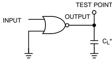
\*Includes all probe and jig capacitance
