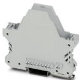
Component housing, length: 99 mm, with vents, Cross connection: integrated bus connector, color: light gray, width: 22.5 mm, height: 92 mm, number of positions cross connector: 10+2
