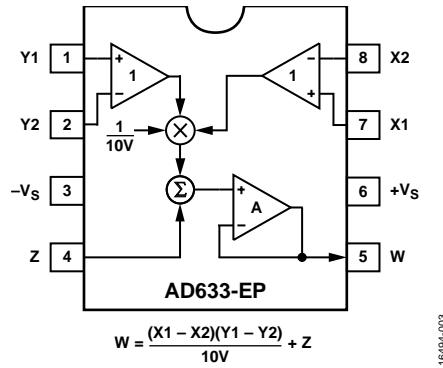
Figure 3. Pin Configuration
