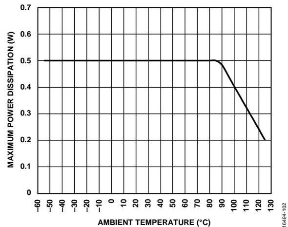
Figure 2. Maximum Power Dissipation vs. Ambient Temperature ( $T_A$ )
