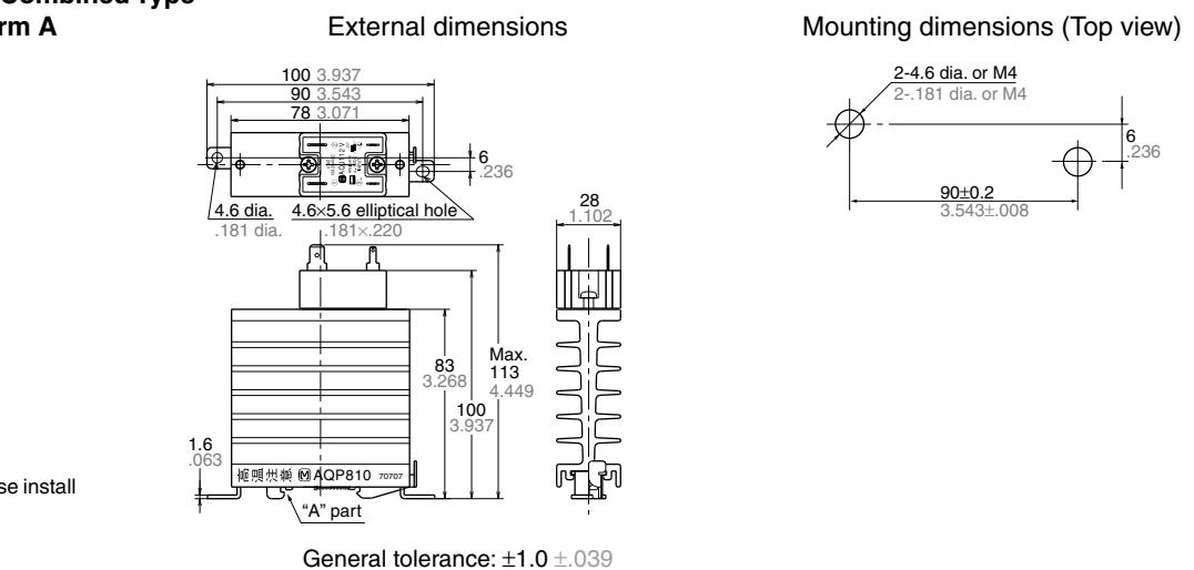
**2.-{(2)} AQ-J Slim Heat Sink Combined Type****Output Arrangement: 1 Form A × 2****CAD**
