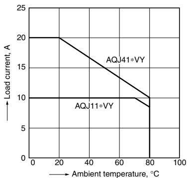
**Use load current within range specified in the figure below**
