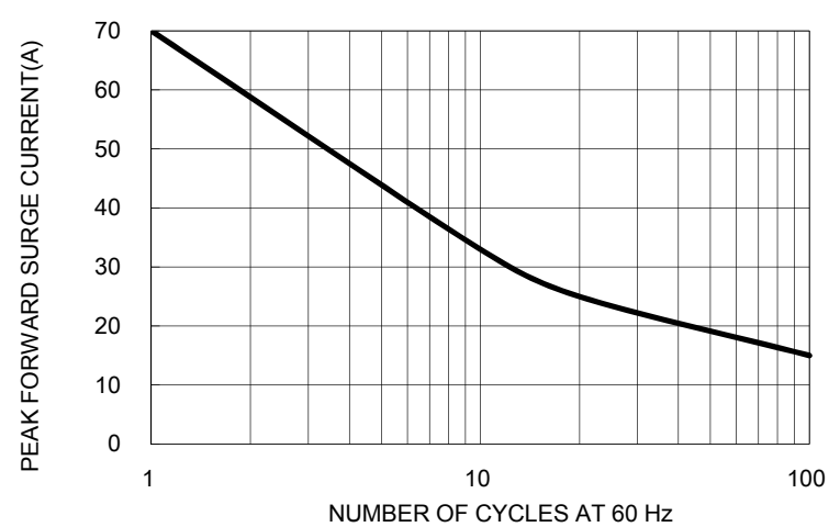
FIG. 2 MAXIMUM FORWARD SURGE CURRENT
