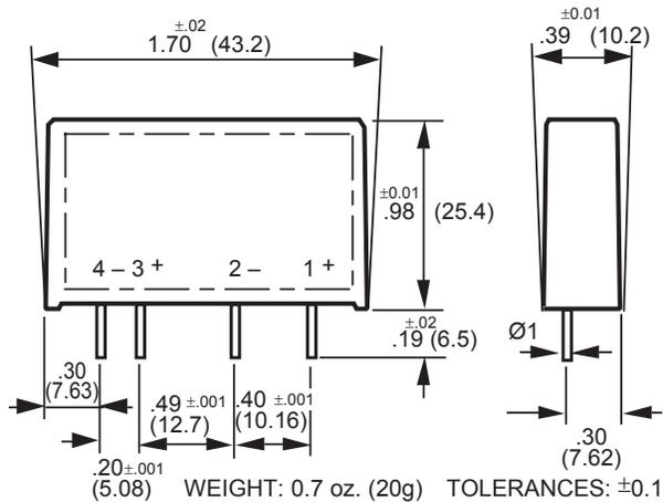
Figure 1 – DS relays; dimensions in inches (mm)
