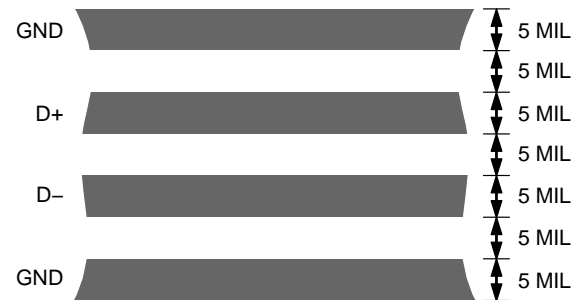
Figure 12. Typical Assignment of Signal Tracks
