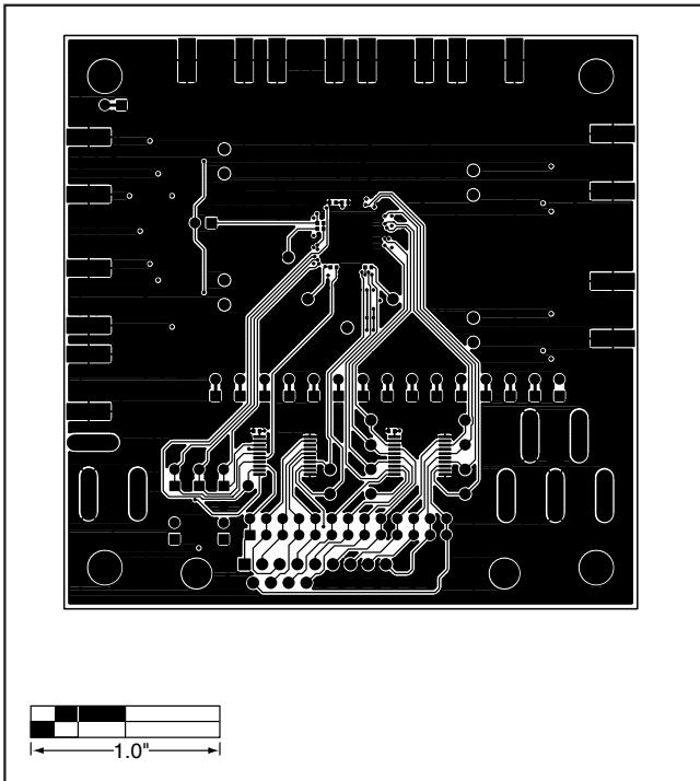
Figure 6. MAX2828/MAX2829 EV Kit PC Board Layout—Solder Side
