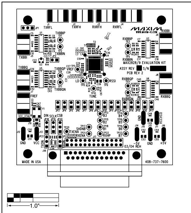
Figure 2. MAX2828/MAX2829 EV Kit PC Board Layout—Top Silkscreen
