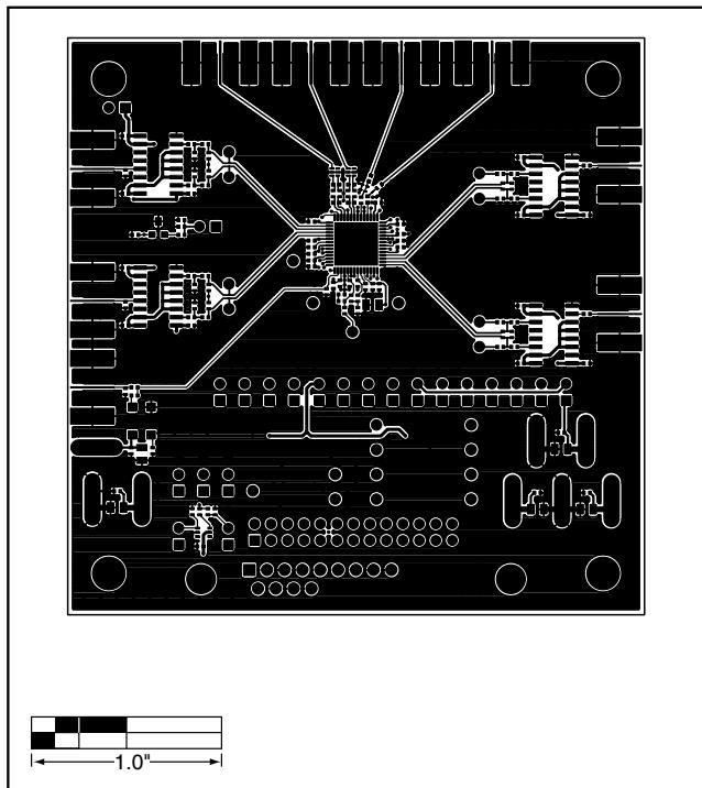
Figure 3. MAX2828/MAX2829 EV Kit PC Board Layout—Component Side
