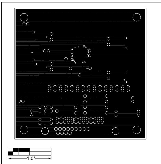
Figure 4. MAX2828/MAX2829 EV Kit PC Board Layout—Inner Layer 2
