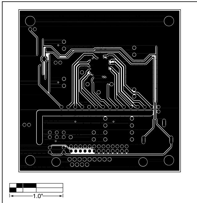
Figure 5. MAX2828/MAX2829 EV Kit PC Board Layout—Inner Layer 3
