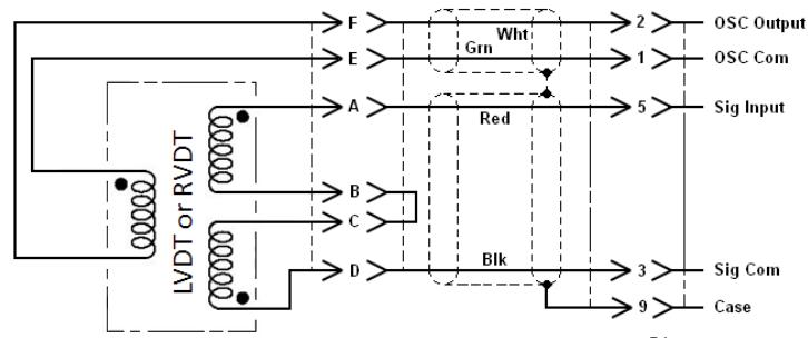
TRANSDUCER WITH CONNECTOR AND JUMPER CABLE
