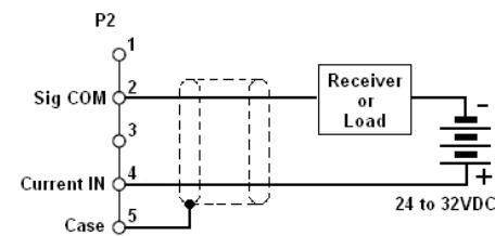
4-20mA OUTPUT USING AN EXTERNAL LOOP SUPPLY
