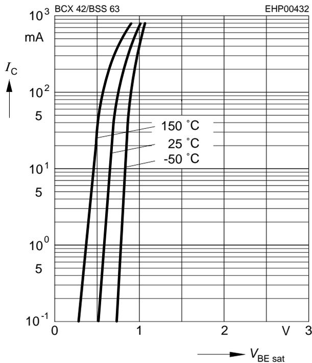
**Collector current  $I_C = f(V_{BE})$**
