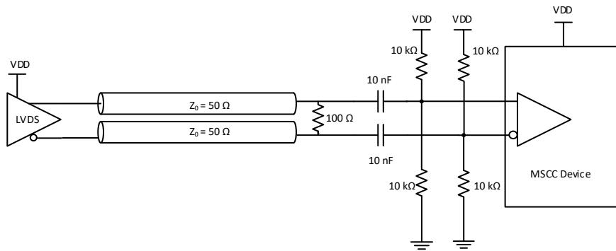
**Figure 9. Input driven by AC coupled LVDS**
