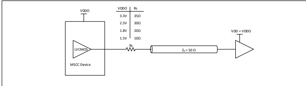
**Figure 11. Termination for LVCMS output**
