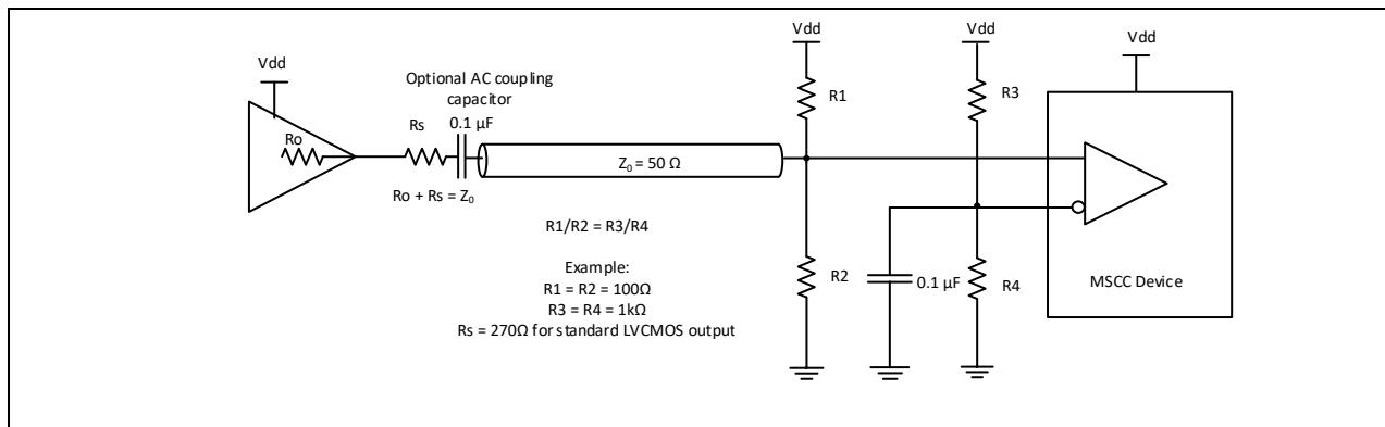
Figure 3. Input driven by a single ended output
