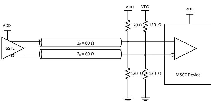
**Figure 10. Input driven by an SSTL output**
