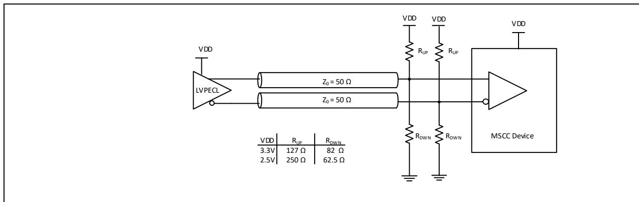
Figure 4. Input driven by DC coupled LVPECL output
