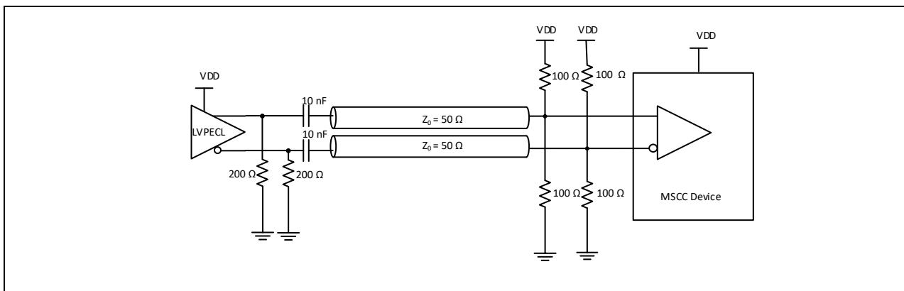
**Figure 6. Input driven by AC coupled LVPECL output**
