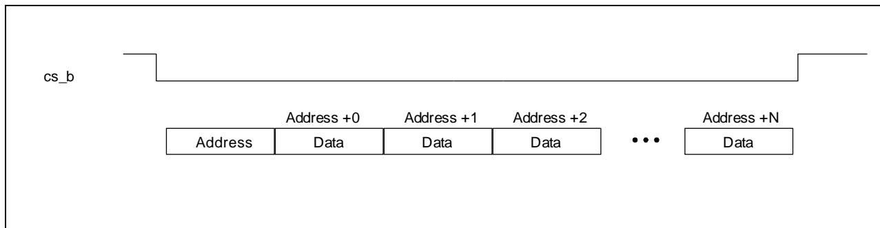
**Figure 18. Example of the Burst Mode Operation**
