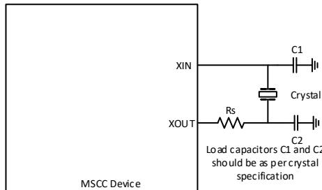
**Figure 13. Crystal Oscillator Circuit in Hardware Controlled Mode**
