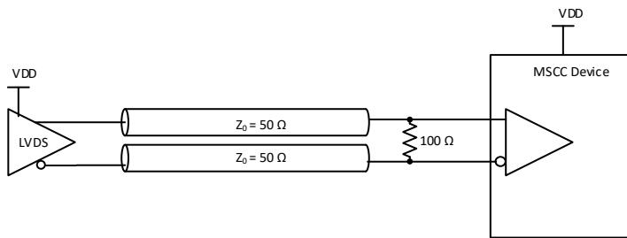
**Figure 8. Input driven by LVDS output**
