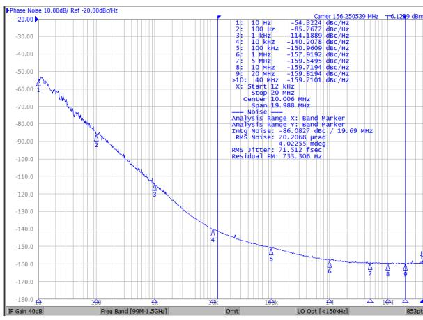
Figure 29. 156.25MHz LVDS Phase Noise in Xtal mode
