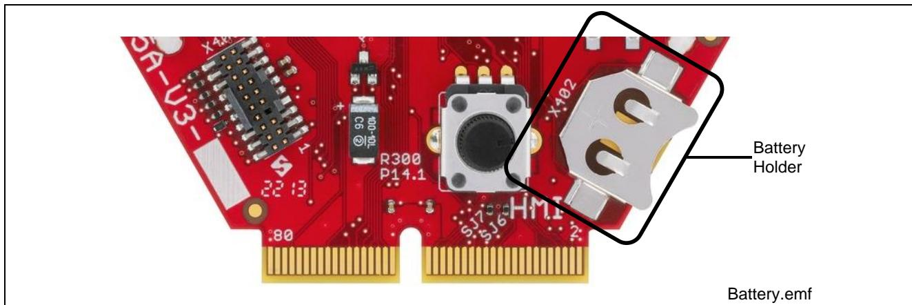
**Figure 19 Battery Holder for Coin Cell**
