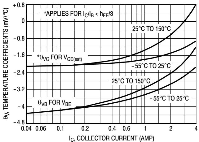
Figure 10. Temperature Coefficients
