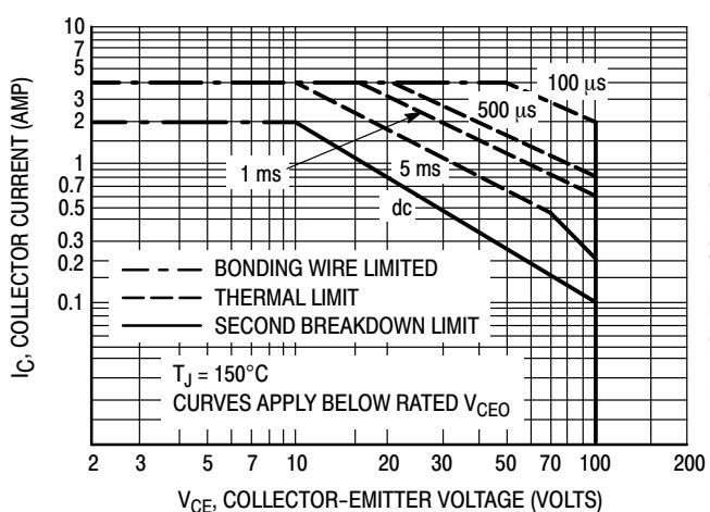
**Figure 4. Maximum Rated Forward Biased Safe Operating Area**
