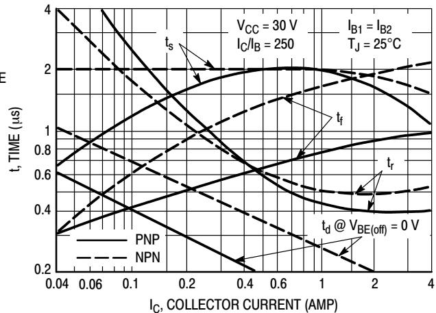
Figure 2. Switching Times
