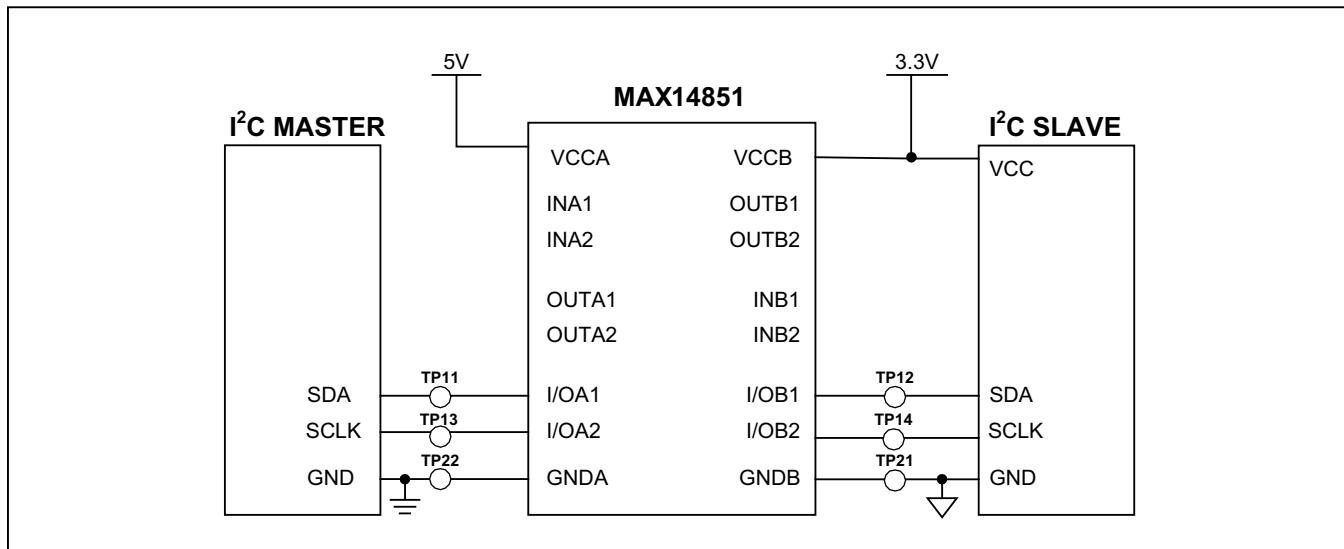
Figure 3. Simplified Connection Diagram for Evaluating the MAX14851 in an Isolated I<sup>2</sup>C Configuration
