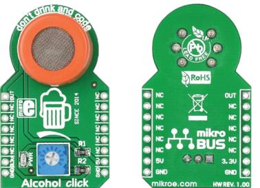
Alcohol click™ is a simple solution for adding a high-sensitivity alcohol gas sensor to your design. The board features an MQ-3 sensor with a SnO<sub>2</sub> gas sensing layer, a calibration potentiometer, a mikroBUS™ host socket, two jumpers and a power indicator LED. Alcohol click™ communicates with the target board through mikroBUS™ AN (OUT) line. Alcohol click™ is designed to use a 5V power supply only.
