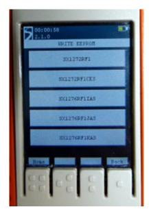
Switch-OFF and ON the Eiger platform to read the new part number from the EEPROM, the firmware will automatically select the right modules settings. Check the Part number of the module plugged on the Eiger platform by clicking on menu ->System->About->Target device.
