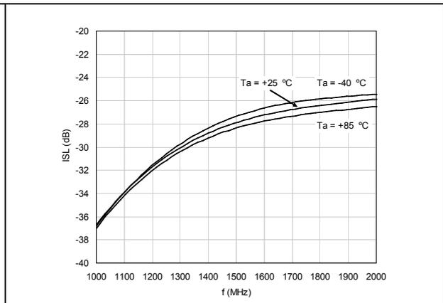
Figure 7. Output return loss vs. frequency
