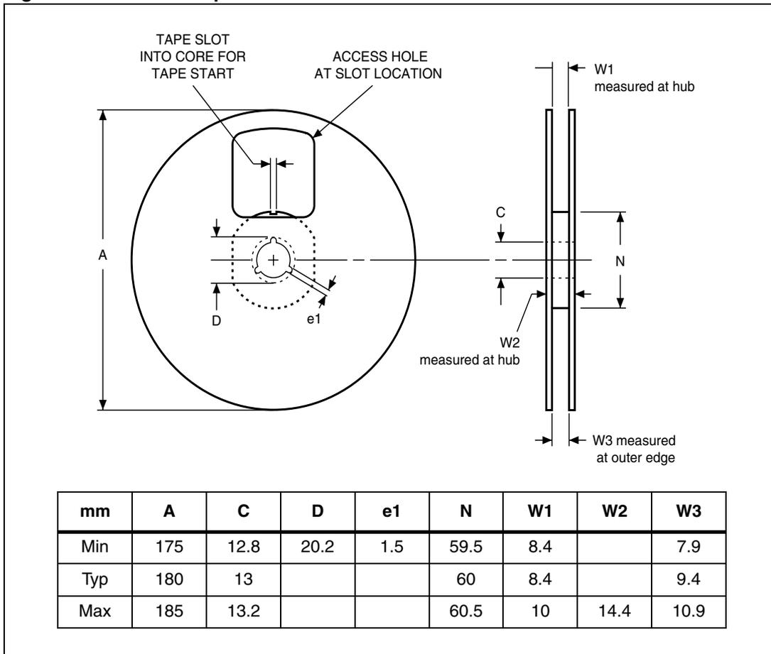
Figure 19. Carrier tape requirements
