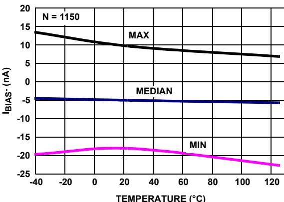
FIGURE 29.  $I_{BIAS^-}$  vs TEMPERATURE,  $V_+, V_- = \pm 1.2V$
