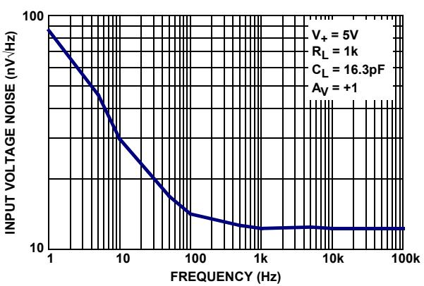
**Typical Performance Curves** $V_+ = 5V, V_- = 0V, V_{CM} = 2.5V, R_L = \text{Open}$  (Continued)
