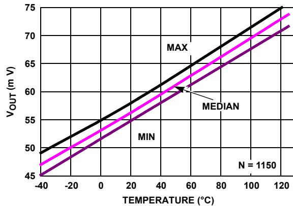
FIGURE 37.  $V_{OUT}$  LOW vs TEMPERATURE,  $V_+, V_- = \pm 2.5V$ ,  $R_L = 1k$ **Pin Descriptions**
