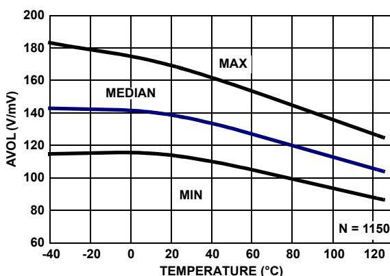
FIGURE 35. AVOL vs TEMPERATURE,  $V_+, V_- = \pm 2.5V$ ,  $V_O = -2V$  TO  $+2V$ ,  $R_L = 1k$
