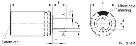
The series B41897 and B41898 have no sleeve nor minus pole marking, the positive pole is marked on the aluminum case side instead.
