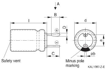
The series B41897 and B41898 have no sleeve nor minus pole marking, the positive pole is marked on the aluminum case side instead.
