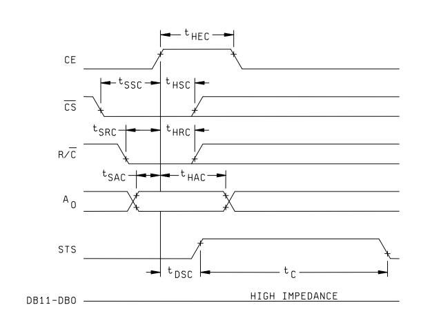
FIGURE 4. Converter start timing diagram.
