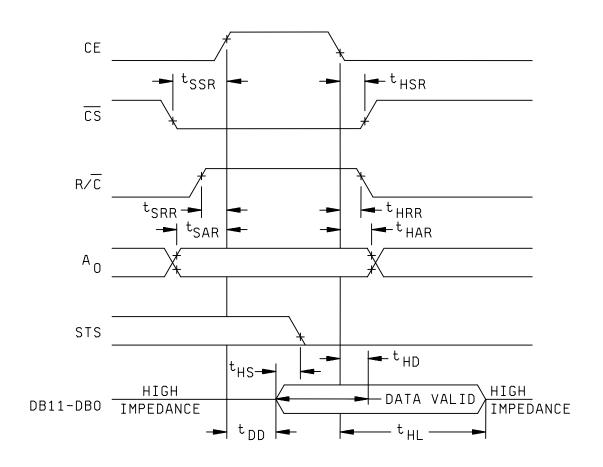
FIGURE 5. Read timing diagram.
