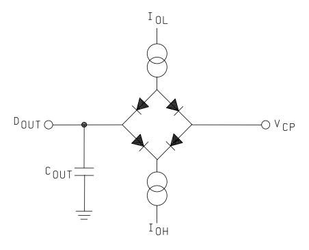
FIGURE 8. Load circuit for bus timing specifications.
