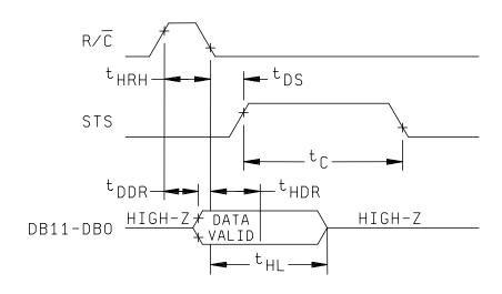
FIGURE 7. Stand-alone mode timing high pulse for  $R/\overline{C}$  diagram.
