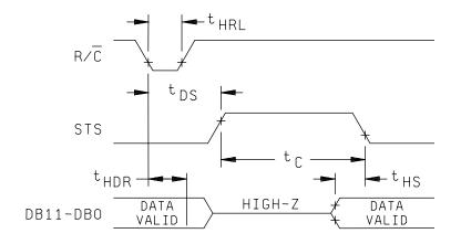
FIGURE 6. Stand-alone mode timing low pulse for  $\mbox{R/}\,\overline{\mbox{C}}\,$  diagram.
