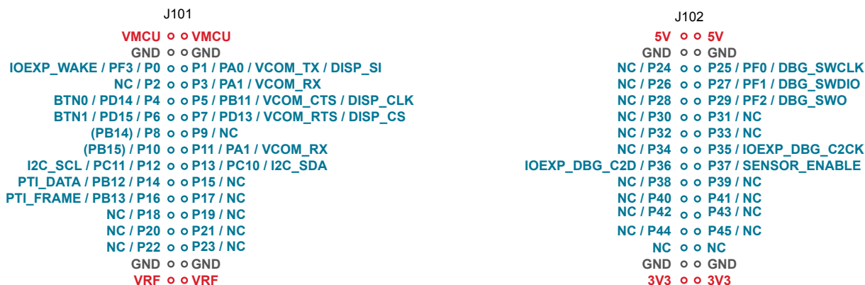
Figure 4.2. Radio Board Pin Mapping on Breakout Pads
