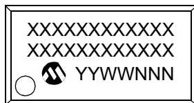
28-Lead SSOP (5.30 mm)
