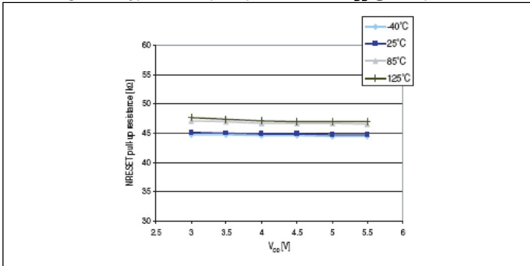
**Figure 34. Typical NRST pull-up current vs  $V_{DD}$  @ 4 temperatures**
