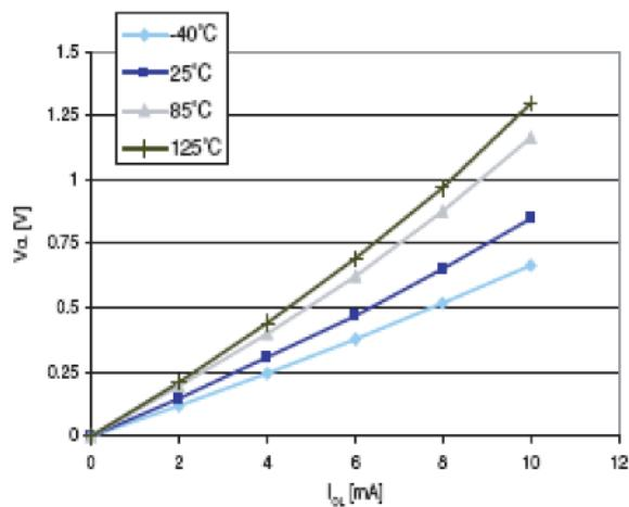
**Figure 23. Typ.  $V_{OL}$  @  $V_{DD} = 3.3 \text{ V}$  (standard ports)**
