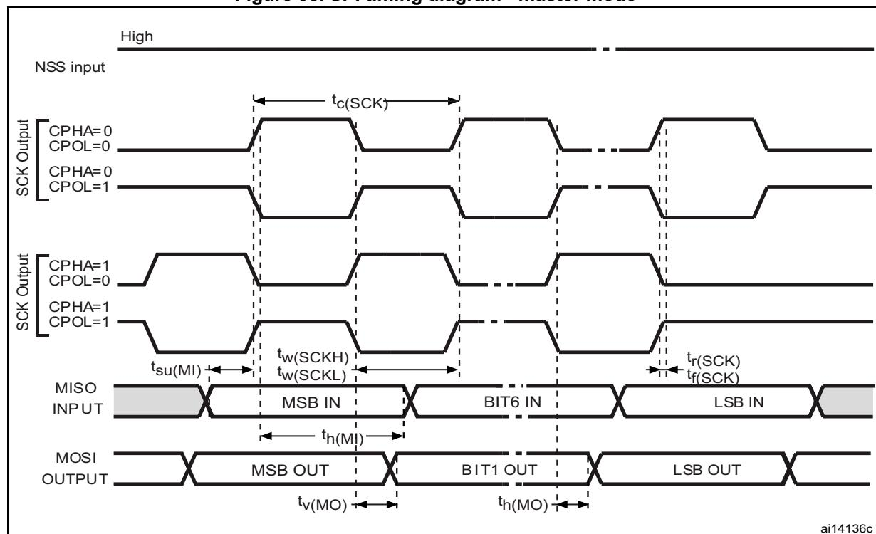
1. Measurement points are at CMOS levels:  $0.3 V_{DD}$  and  $0.7 V_{DD}$ .
