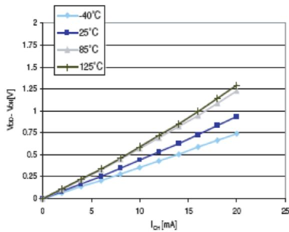
**Figure 31. Typ.  $V_{DD} - V_{OH}$  @  $V_{DD} = 3.3$  V (high sink ports)**
