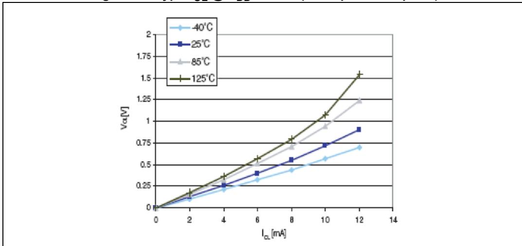
**Figure 26. Typ.  $V_{OL}$  @  $V_{DD} = 5$  V (high sink ports)**
