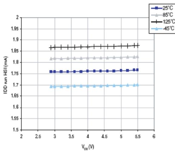
**Figure 14. Typ  $I_{DD(WFI)}$  vs.  $V_{DD}$  HSE user external clock,  $f_{CPU} = 16$  MHz**
