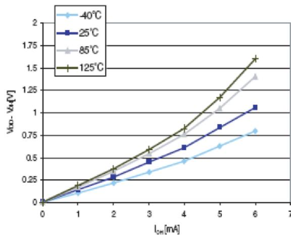
**Figure 29. Typ.  $V_{DD} - V_{OH}$  @  $V_{DD} = 3.3$  V (standard ports)**
