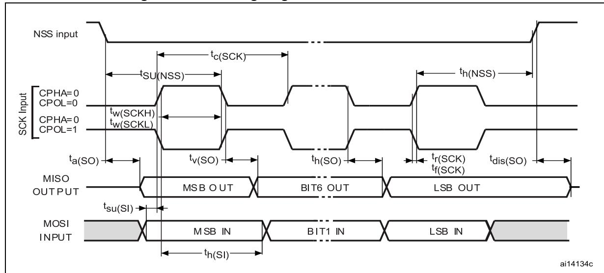
1. Measurement points are made at CMOS levels: 0.3  $V_{DD}$  and 0.7  $V_{DD}$ .
