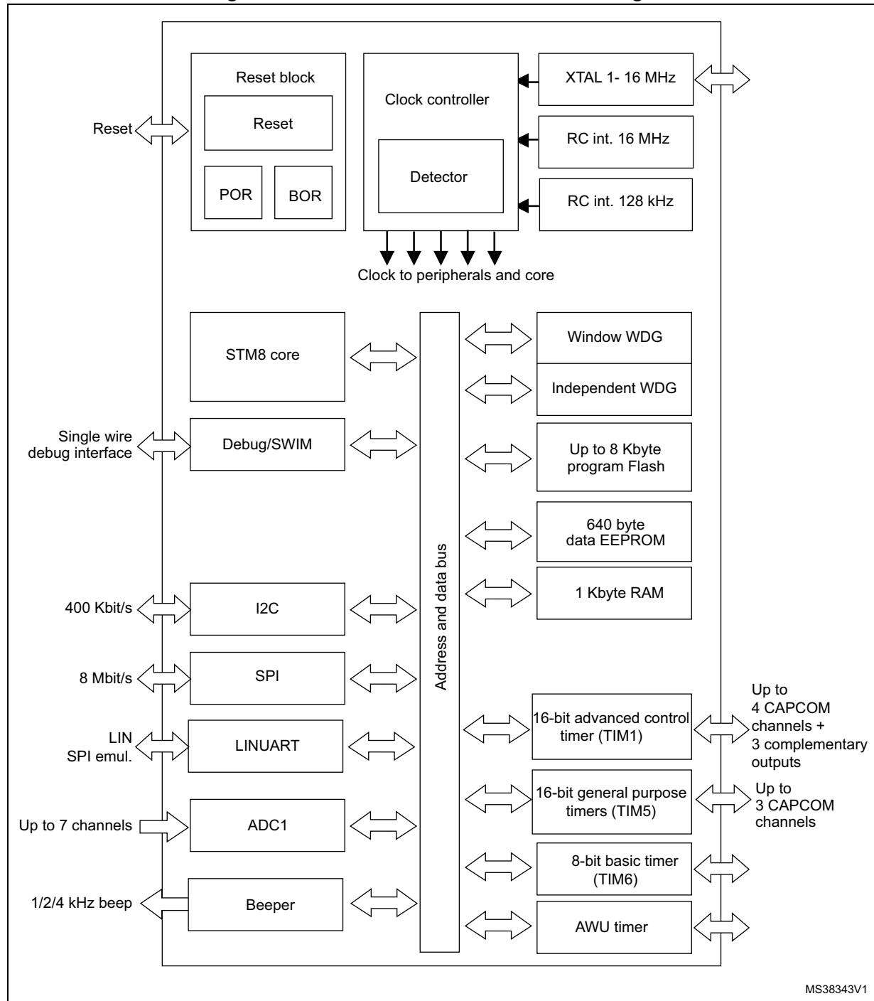
1. **Legend:** ADC (Analog-to-digital converter), beCAN (Controller area network), BOR (Brownout reset), I<sup>2</sup>C (Inter-integrated circuit multimaster interface), IWDG (Independent window watchdog), LINUART (Local interconnect network universal asynchronous receiver transmitter), POR (Power on reset), SPI (Serial peripheral interface), SWIM (Single wire interface module), USART (Universal synchronous asynchronous receiver transmitter), Window WDG (Window watchdog).
