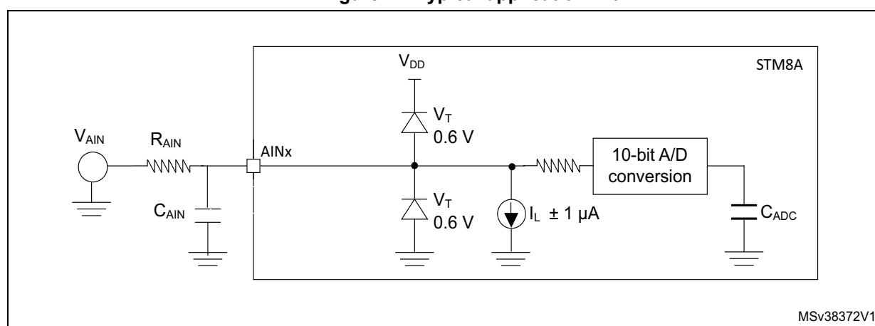
1. Legend:  $R_{\text{AIN}}$  = external resistance,  $C_{\text{AIN}}$  = capacitors,  $C_{\text{samp}}$  = internal sample and hold capacitor.
