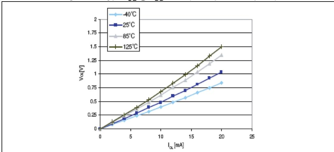
**Figure 25. Typ.  $V_{OL}$  @  $V_{DD} = 3.3$  V (true open drain ports)**
