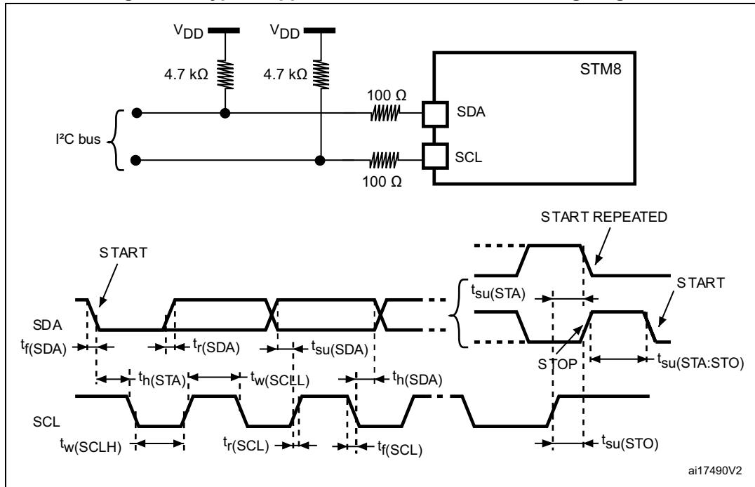
1. Measurement points are made at CMOS levels:  $0.3 \times V_{DD}$  and  $0.7 \times V_{DD}$ .
