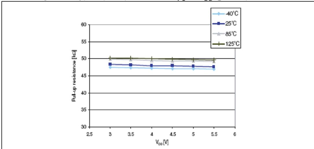
Figure 21. Typical pull-up current  $I_{pu}$  vs  $V_{DD}$  @ 4 temperatures
