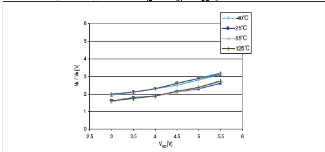
Figure 33. Typical NRST pull-up resistance vs  $V_{DD}$  @ 4 temperatures
