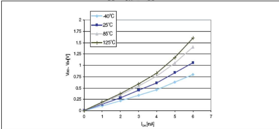
Figure 29. Typ.  $V_{DD} - V_{OH}$  @  $V_{DD} = 3.3$  V (standard ports)
