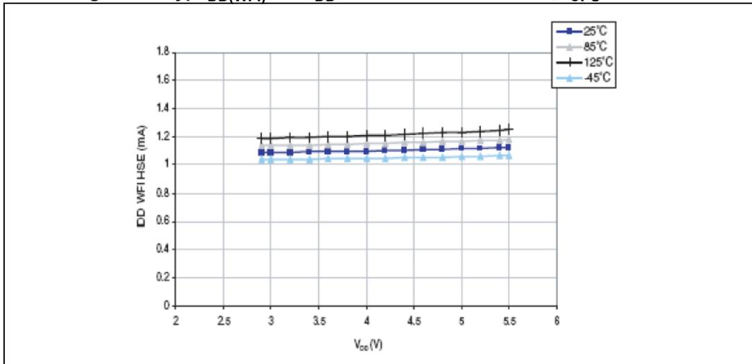
Figure 15. Typ  $I_{DD(WFI)}$  vs.  $f_{CPU}$  HSE user external clock,  $V_{DD} = 5\text{ V}$
