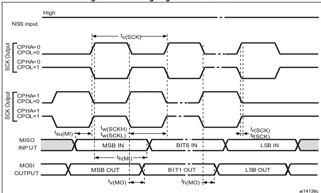
1. Measurement points are at CMOS levels: 0.3 V<sub>DD</sub> and 0.7 V<sub>DD</sub>.
