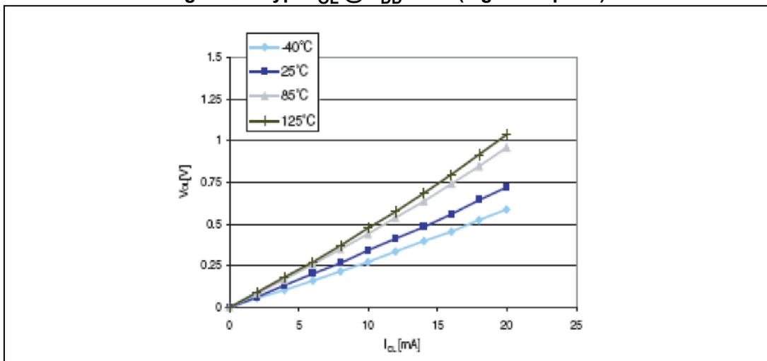
Figure 27. Typ.  $V_{OL}$  @  $V_{DD} = 3.3$  V (high sink ports)
