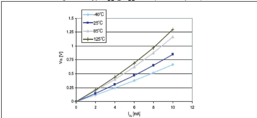
Figure 23. Typ. V<sub>OL</sub> @ V<sub>DD</sub> = 3.3 V (standard ports)
