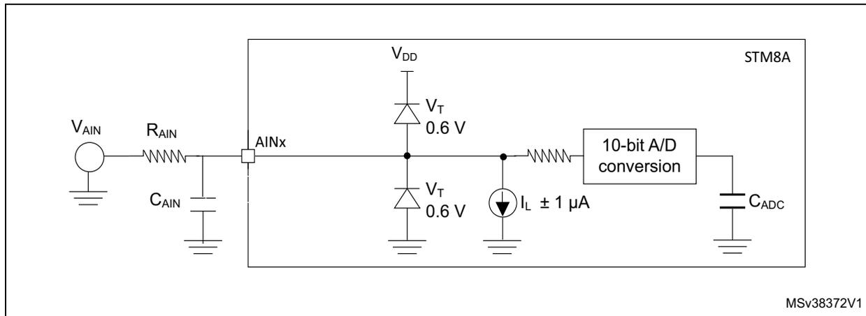
1. Legend: R<sub>AIN</sub> = external resistance, C<sub>AIN</sub> = capacitors, C<sub>samp</sub> = internal sample and hold capacitor.
