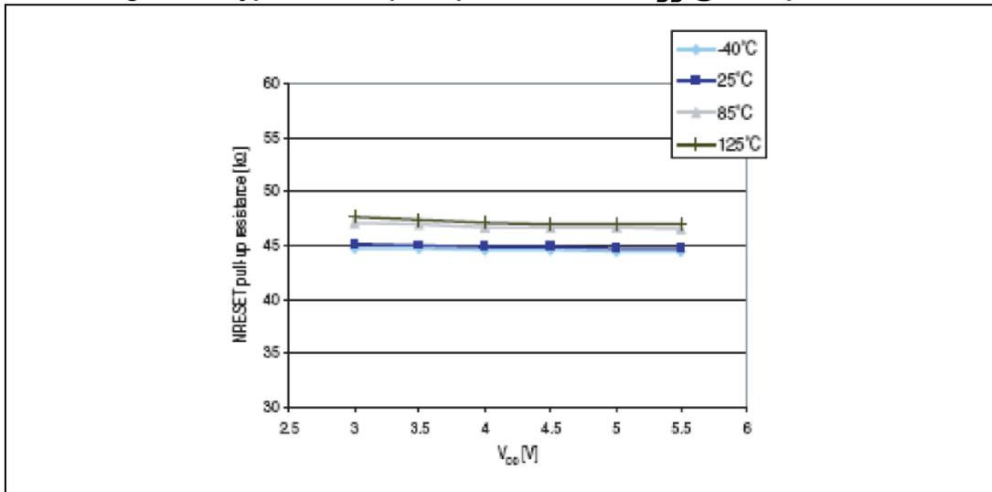
Figure 34. Typical NRST pull-up current vs  $V_{DD}$  @ 4 temperatures
