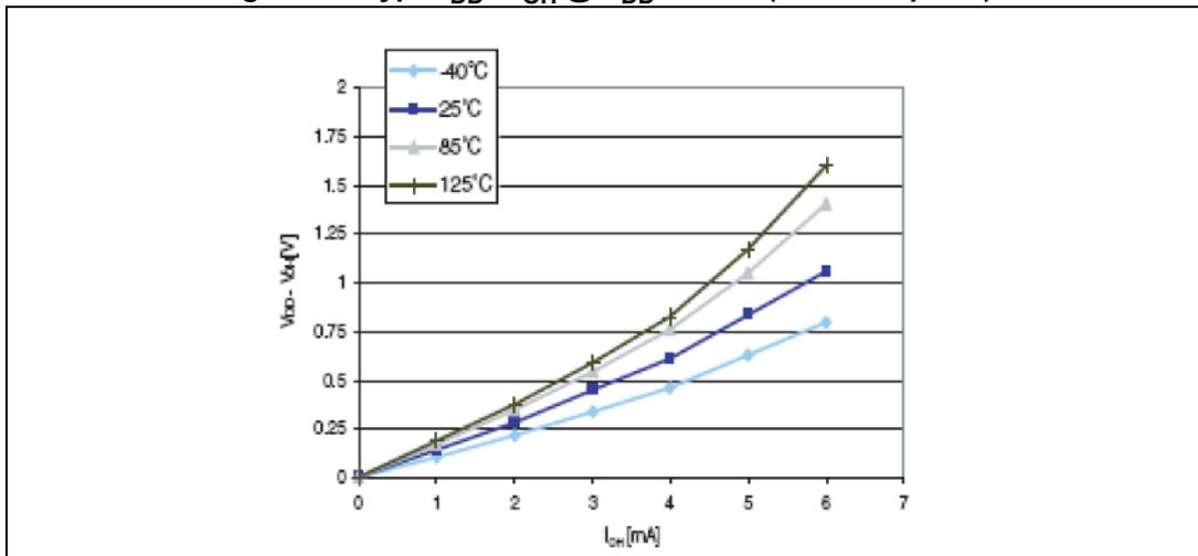
Figure 30. Typ.  $V_{DD} - V_{OH}$  @  $V_{DD} = 5\text{ V}$  (high sink ports)
