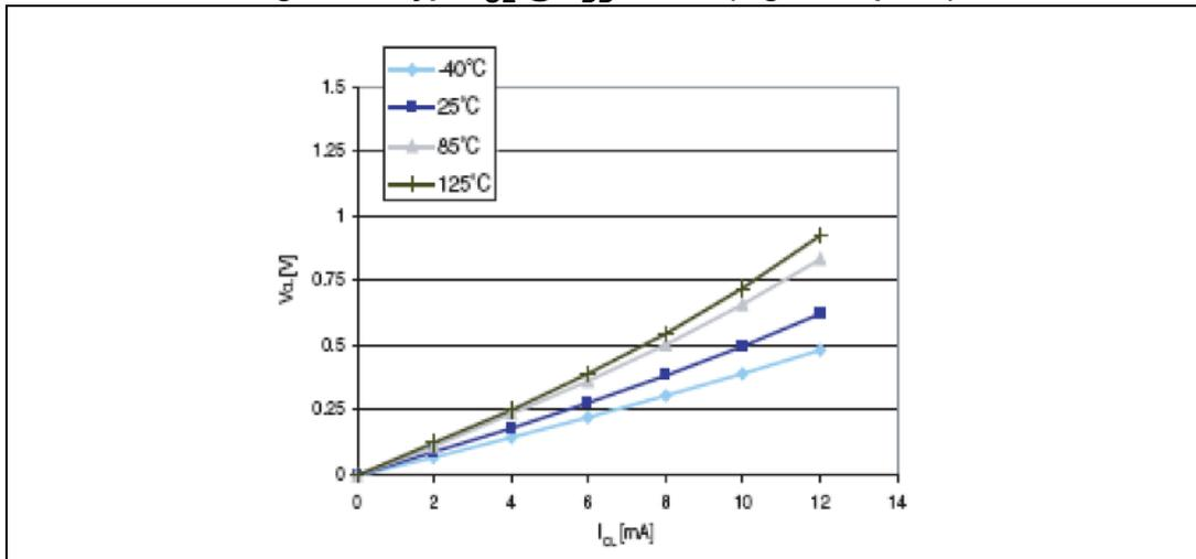
Figure 28. Typ.  $V_{DD} - V_{OH}$  @  $V_{DD} = 5$  V (standard ports)
